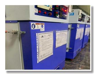
Thermal aging is used to test the ability of a product to with stand elevated temperatures for an extended period of time. This test measures the change in LLCR and mating / un-mating force both before and after the parts have been thermally exposed in a thermal chamber.
